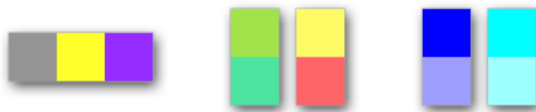
Figure 1: Examples of non perceptual uniformity in HLS. Left: Three colors of equal lightness. Middle: Two pairs of colors with equal hue distance. Right: Two pairs of colors with equal lightness distance.
